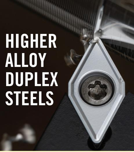
Higher alloy duplex steels are known for being difficult to machine – especially when it comes to heat generation, cutting forces and chip control – higher alloy duplex steels require optimized chip control and coolant to avoid plastic deformation.
